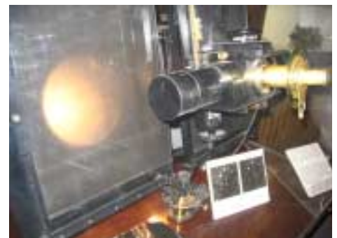
The last planet discovered – Pluto, was discovered in 1930 using this device, the blink comparator. It is used to compare two images taken at different times.
